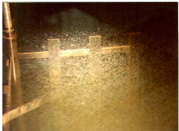
Coagulation with Ferric Sulfate: Little Rock, AR
