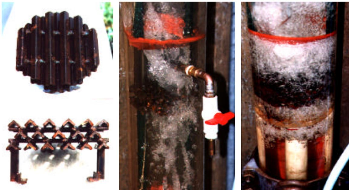
**Iron Column Packing Grates used in Tower Aerator under Free-Fall and Submerged Conditions**
