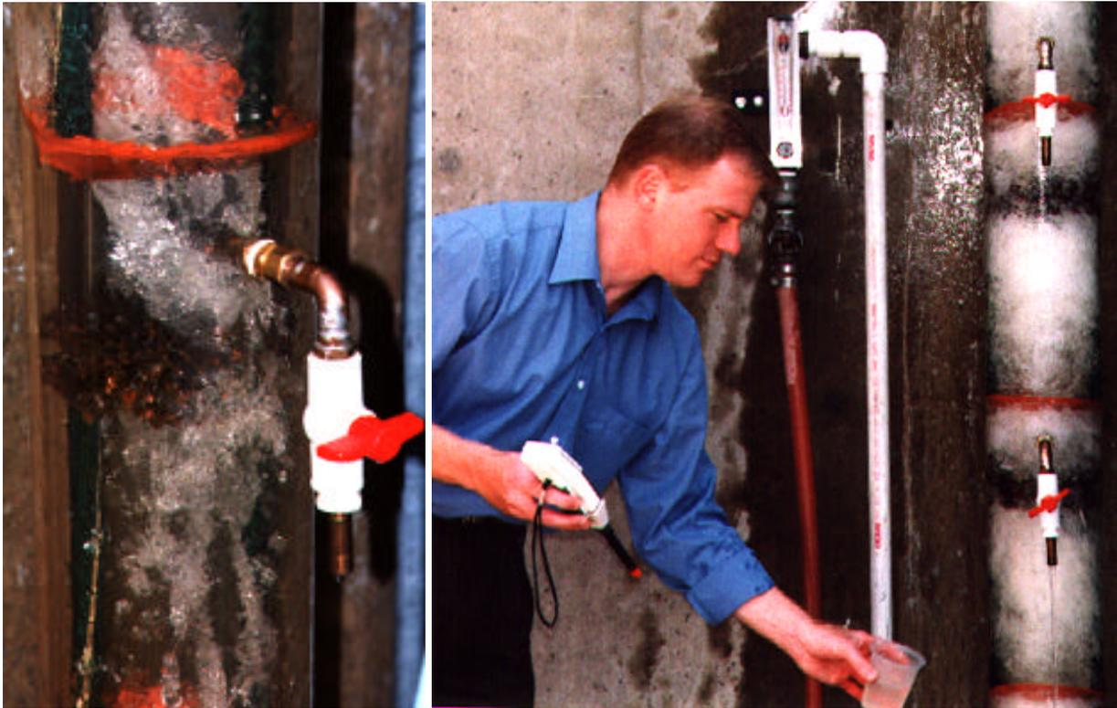
**Operation and Sampling of Tower Aerator under Free-Fall with Iron Grate Packing**
