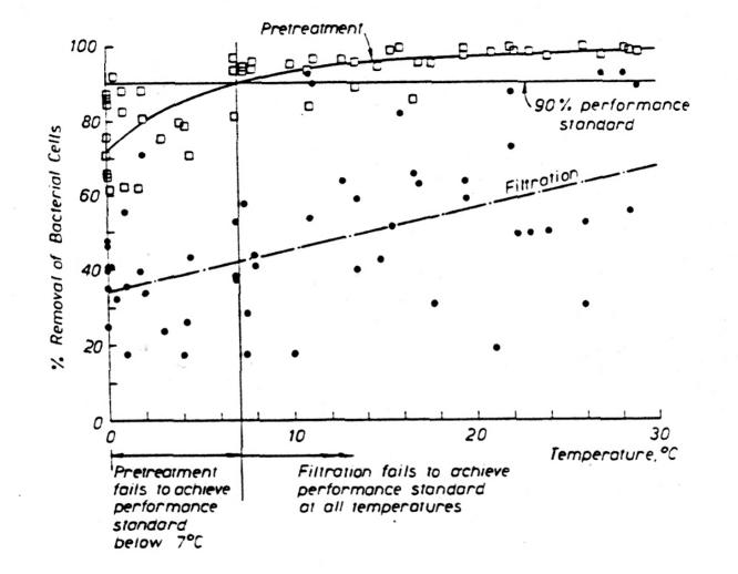
FIG. 2 -- Effect of temperature on removal of bacterial cells by pretreatment and filtration
