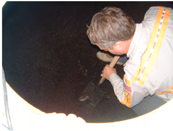
Filter media probing and sampling were conducted on November 18, 2002.
