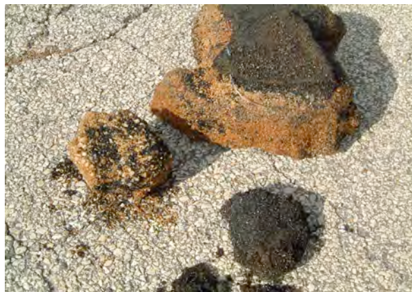
Most of the severely cemented (sandy) material appeared to underlie the coal layer. The coal media also showed evidence of a loose aggregation that could be broken up by hand.
